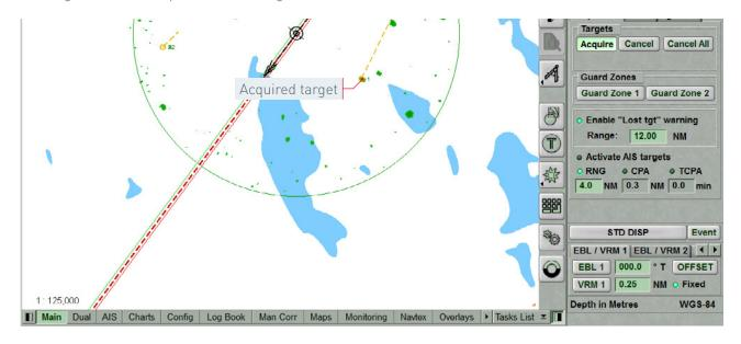
If you press the right trackball button, the cursor exits from the target acquisition mode.
