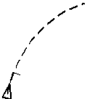
AIS target turning starboard, ROT is measured by ROT gyro
