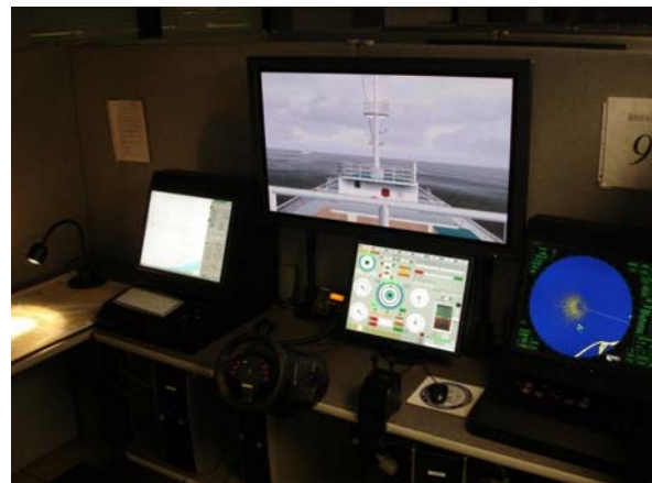
Figure 2 16-workstation Integrated Navigation Lab (INL) for solo ECDIS navigation and assessment
